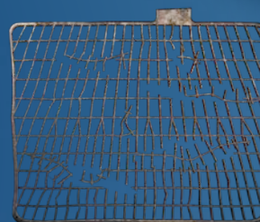
STANDARD GRID shown after 50,000 KM corrosion
